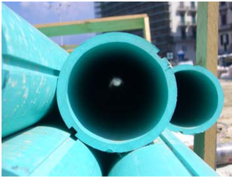
Fig 4: The pipe used to mount the coil. You can see clearly the indents down both sides, which were used to align the cable accurately along the coil's entire length.
